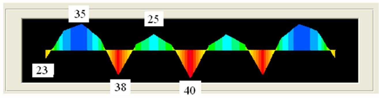
bending moment in slab KN.m
