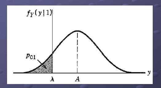
The probability of error that symbol 1 is sent and received bit is mistakenly read as 0 is given by
