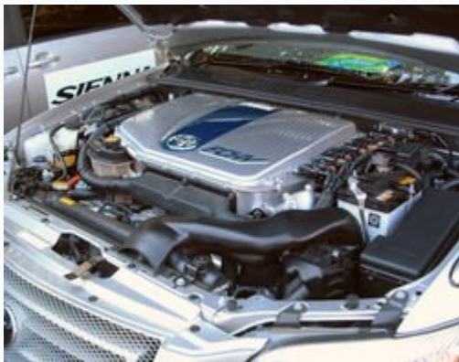
Toyota FCHV PEM FC fuel cell vehicle
