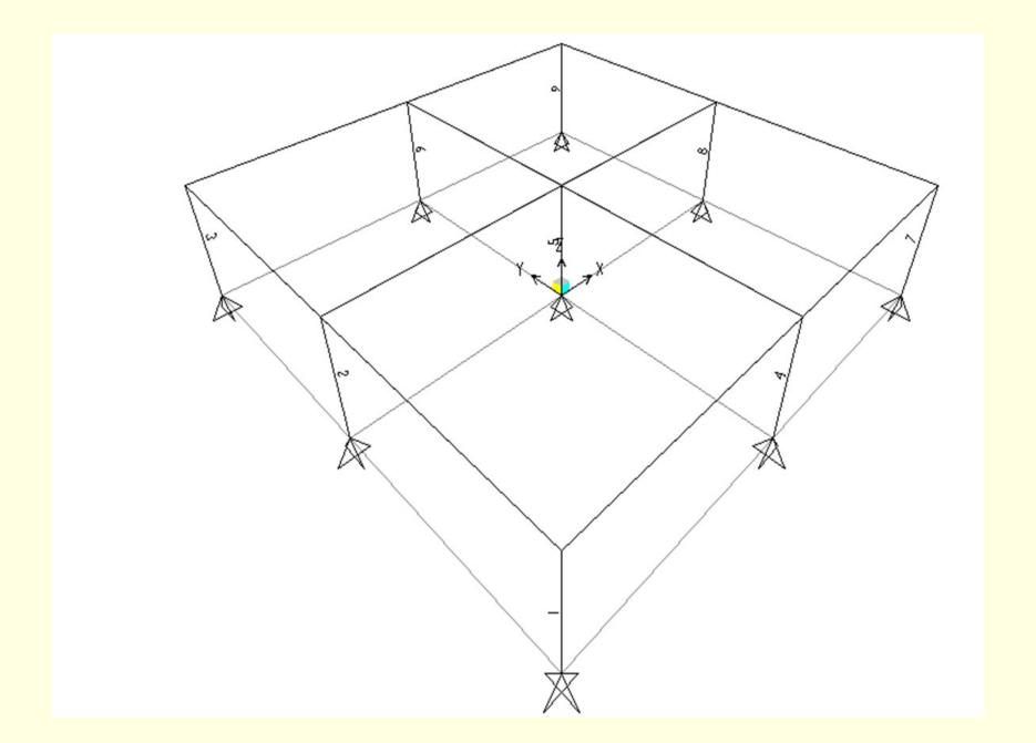
a one-story flat plate reinforced concrete building subjected to earthquake loading in the x-direction. The thickness of slab is 20cm, columns are square having 40cm dimensions, 3m elevation and the distance between them is 6m.
