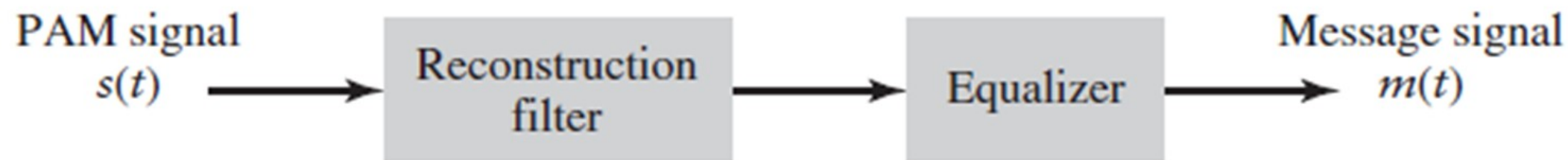
FIGURE 5.7 Recovering the message signal m(t) from the PAM signal s(t) .
