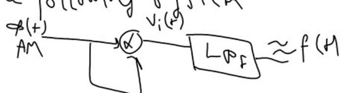
$$\begin{aligned} V_i(t) &= \phi_{AM}^2(t) \\ &= \left[ A(1+mf(t)) \cos\omega_ct \right]^2 \\ &= A^2(1+2mf(t)+m^2f^2(t)) \cos^2\omega_ct \\ &= \frac{1}{2}A^2(1+2mf(t)+m^2f^2(t)) + \\ &\quad \frac{1}{2}A^2(1+2mf(t)+m^2f^2(t)) \cos 2\omega_ct \end{aligned}$$
