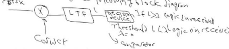
Note the BPSK demodulator is in fact a synchronous (coherent) detector, therefore it requires a synchronization circuit between the transmitter and the receiver.
