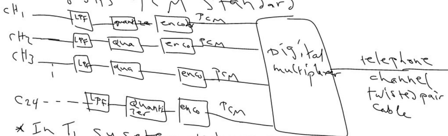
\* In T<sub>1</sub> system we have 24 samples each sample is represented by 8 bits so the total number of bits per sample (frame) is equal  $8 \times 24 = 192$  bits/frame
