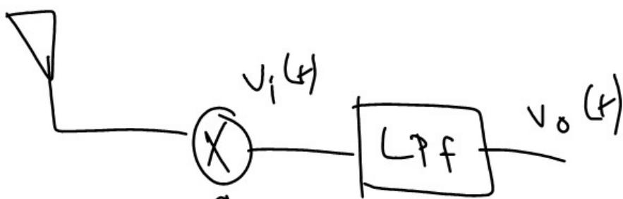
$$\begin{aligned} V_i(t) &= f(t) \cos \omega_c t \cos(\omega_c t + \theta_0) \\ &= f(t) \left[ \frac{1}{2} \cos(2\omega_c t + \theta_0) + \frac{1}{2} \cos \theta_0 \right] \end{aligned}$$
