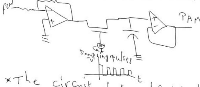
\* The circuit that can be used to generate natural samples is shown below
