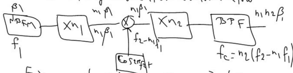
Ex for the indirect FM modulator shown above assume  $f_1 = 200\text{kHz}$ ,  $f_2 = 10.8\text{MHz}$ ,  $n_1 = 64$  and  $n_2 = 48$ . Determine the possible carrier frequencies at the modulator output and the peak frequency deviation if the peak frequency deviation of the NBFM = 25 Hz
