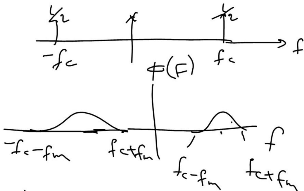
\* Note that the previous amplitude modulation is called double side band because the bandwidth required for the transmission of the modulated signal is  $BW = (f_c + f_m) - (f_c - f_m) = 2f_m$  (doubled)
